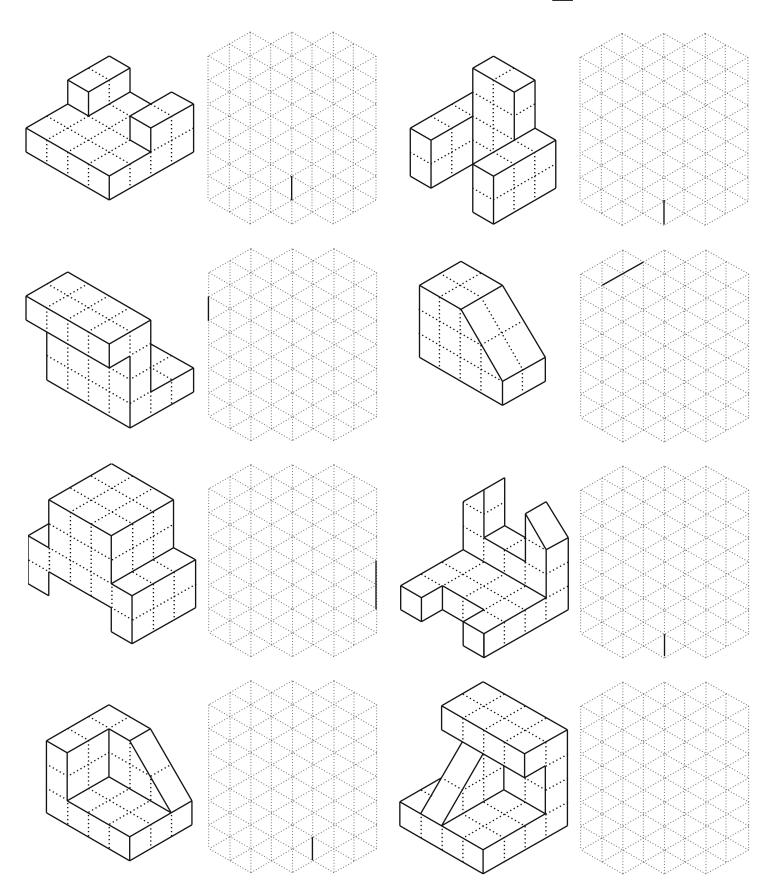
**Basic Isometric Drawing I and II**Please redraw the shapes. Use the dotted lines to assist and guide you.
