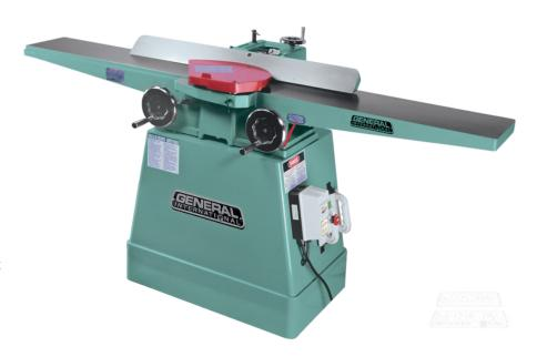
Never joint or plane a piece of stock that is shorter than 250 mm (10"), narrower than 19 mm (3/4"), or less than 13 mm (1/2") thick. The maximum depth of cut is 3 mm (1/8").
