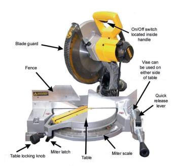
Make certain the blade rotates in the correct direction and that the teeth at the bottom of the blade are pointing to the rear of the miter saw.
