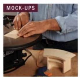
An easy way to test designs. With a scroll saw, small, intricate pieces are easy to cut quickly and assemble using hot-melt glue. This ½o-scale model is a reading podium.
