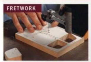
**Endless options for pierced work.** Schürch made this jewelry-box tray by cutting out small openings in solid wood and laying that fretwork onto a felt-covered plywood bottom. He detailed the carved leaf after the main vertical cuts were done.
