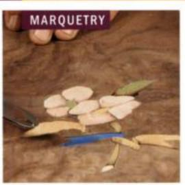
**Indispensable for marquetry.** A scroll saw can cut through a thick packet of veneers (facing page) with a very thin blade, cutting out all of the pieces for a picture in one shot.
