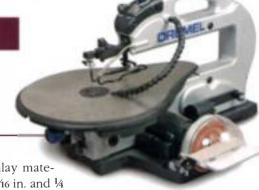
the design onto the inlay material—usually between 1/16 in. and 1/4 in. thick—and cut it out on a scroll saw
