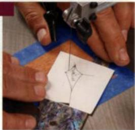
directly to a top piece. On period furniture, I've used a scroll saw to cut out carving blanks for applied decorative elements.
