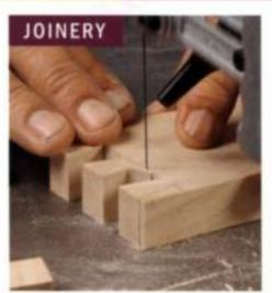
**Perfect for dovetails.** After the initial cheek cuts are made, the tiny scroll-saw blade makes it easy to cut across the bottom of a dovetail socket and quickly remove the waste.
